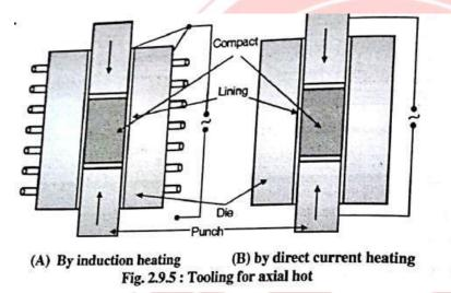
But the process is operated at higher temperature, and pressure. The ceramic powder with the binder are fed into die and pressed at high temperature and pressure into article, followed by sintering and finishing. The temperature can be raised by direct current of induction current.
